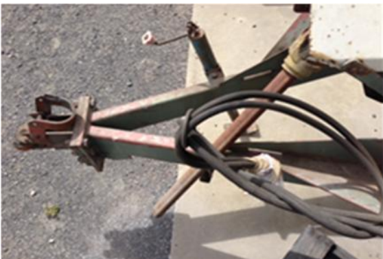
PTO guard missing
