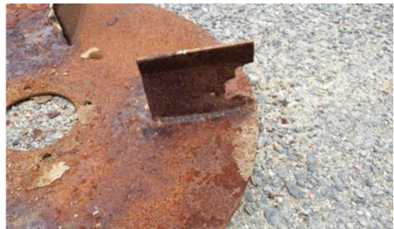
Worn spinner vane tips
