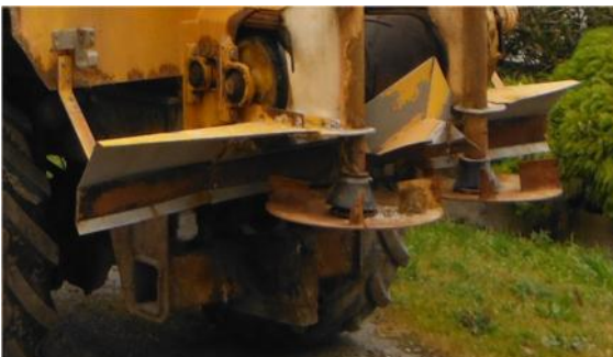
Worn spinner vane tips
